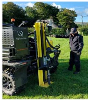
Soil Sampling to one metre deep
