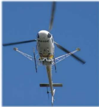
Aerial LiDAR Survey at 15 scans per metre
